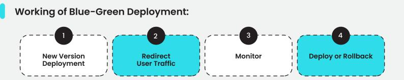
**New Version Deployment:** The process starts by deploying the new version or updates of the software or application into the inactive green environment. This deployment involves installing, configuring, and thoroughly testing the latest version to ensure its proper functionality.
